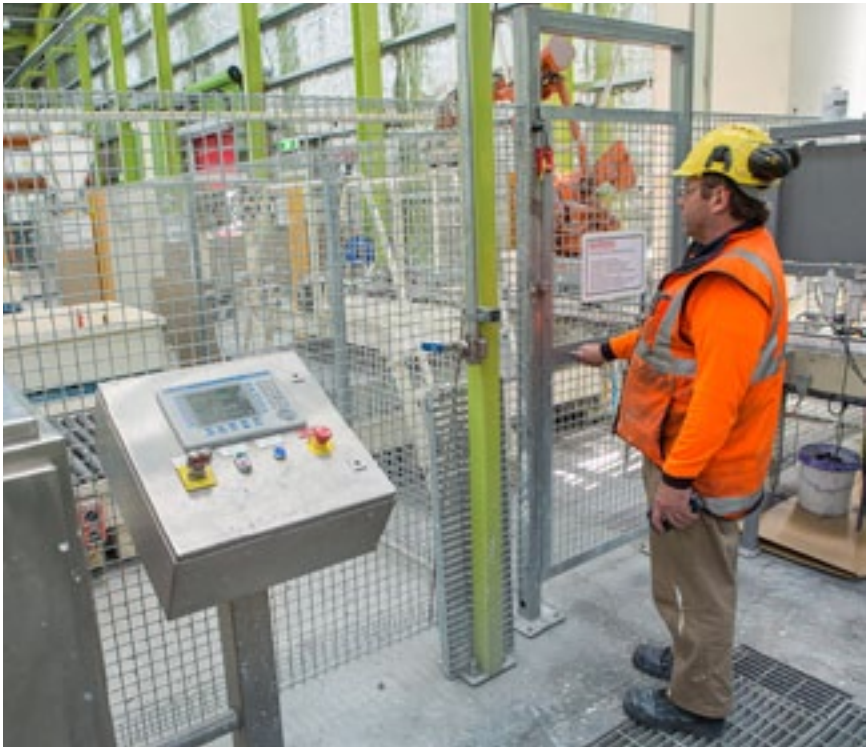
Figure 3: The height of guarding and the dangerous part determines the distance of the guard from the dangerous part.
